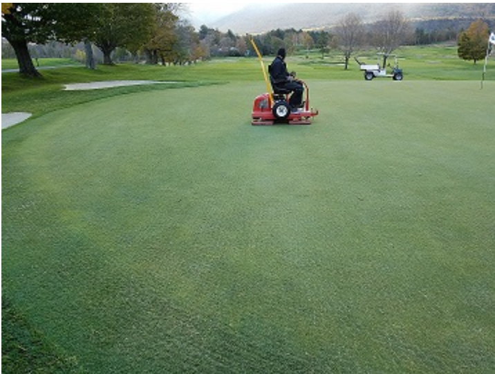
Figure 6-7. Rolling putting green surfaces can allow managers to reduce mowing frequency or raise mowing heights while maintaining putting green speeds.
